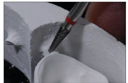
Separating the restoration with cross-cut tungsten carbide burs or other suitable grinding instrument
